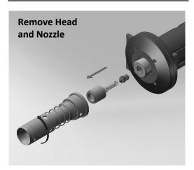
Remove head assembly by rotating in direction of arrow.
