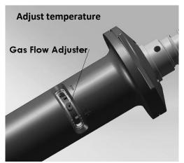
Rotate adjuster towards (+) position to increase gas flow and temperature. Ensure gas flow is smooth and not pulsing.
