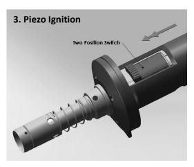
To ignite, push switch forward in direction of arrow to gas on (Pos.1) and then forward again to ignition (Pos.2).
