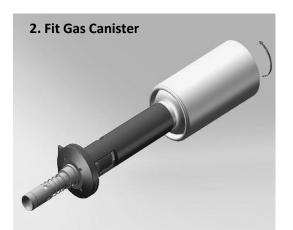
Fit universal Butane Propane Mix (70/30) (EN 417 threaded type) gas canister by rotating in direction of arrow. Ensure seal is made. Do not over tighten. Gas canister can be left on unit when not in use.
