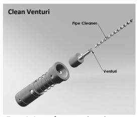
To optimise performance clean the venturi regularly by pushing a pipe cleaner through the centre and cross holes. Visually inspect.
