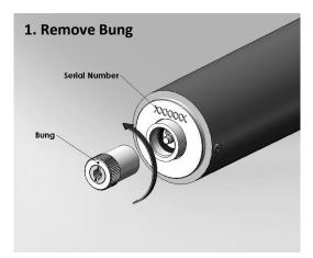
Remove bung by rotating in direction of arrow.
